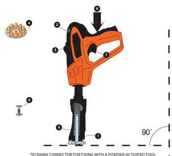
TECNARIA CONNECTOR FOR FIXING WITH A POWDER-ACTUATED TO with separate nails
