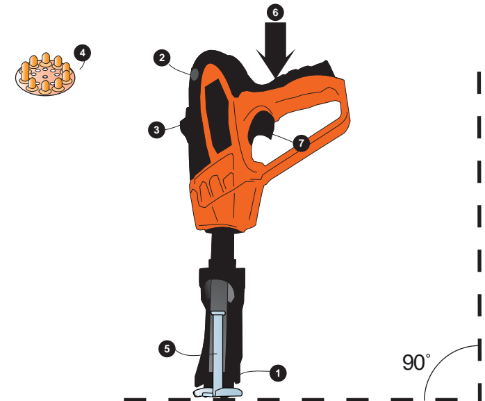
TECNARIA CONNECTOR WITH PRE-ASSEMBLED NAILS FOR FIXING WITH A POWDER-ACTUATED TOOL
