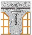
CT CEM stud connector with screw and toothed plate, base 60x50 mm, screw Ø 14 mm
